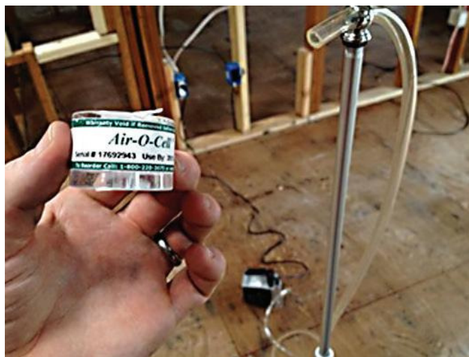
Collecting a post-remediation spore trap air sample – Photo by IAQ Technologies, Inc.
