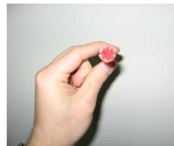
*The tip of an activated LeadCheck swab before and after contact with a surface coated with lead paint*
